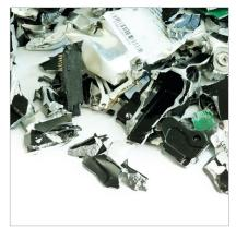
Particles of shredded hard drives Cutting size: 1.5" Security level: H-3
