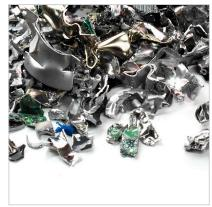
Particles of shredded hard drives Cutting size: 0.39" x 1"-1.18" max Security level: H-5
