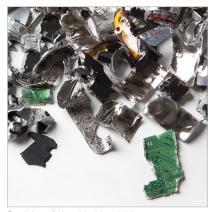
Particles of shredded hard drives Cutting size: 0.78" x 1.57"-2" max Security level: H-4
